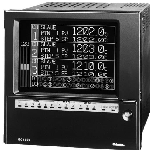
**■ Multiple control of up to 3 channels per single unit**
