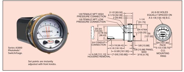
Photohelic® Switch/Gages function as versatile, highly repeatable pressure switches combined with a precise pressure gage employing the time-proven Magnehelic® gage design. The Photohelic® gage measures and controls positive, negative or differential pressures of air and compatible gases. Standard models are rated to 25 psig (1.7 bar) with options to 35 (2.4) or 80 (5.5 bar) psig. Single pressure 36000S models measure to 6000 psig (413 bar) with a 9000 psig (620 bar) rating.
