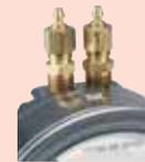
**A-314 Bleed Fitting** — For easier, safer purging of trapped air when using gage with liquids. Also useful for draining condensate when installed in lower ports. To open, simply loosen hex nut. Solid brass.
